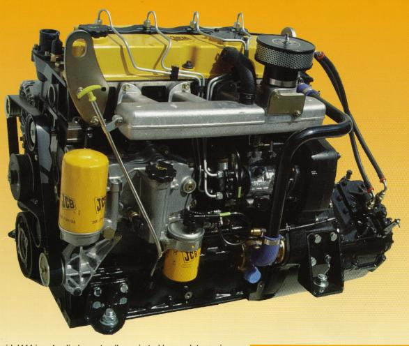
The Mermaid J444 is a 4 cylinder, naturally aspirated heavy duty marine diesel engine and is based on the highly reliable JCB 444 series industrial engine. The engine is suitable for all commercial duties and with the optional gear driven hydraulic pump is particularly suited to inshore fishing vessels and small workboats.
